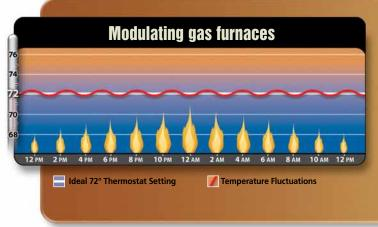
The Coleman® Echelon™ modulating gas furnace has been designed to maintain your ideal temperature by modulating heating level in .50 or .65% increments to match the degree of comfort you need precisely. Comfort is dramatically increased as the furnace adjusts its level of operation up or down to offset the rate at which heat leaves your home.
