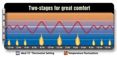
Two-stage gas furnaces offer an immediate level of performance. Operation varies between first and second stage based on demand.
